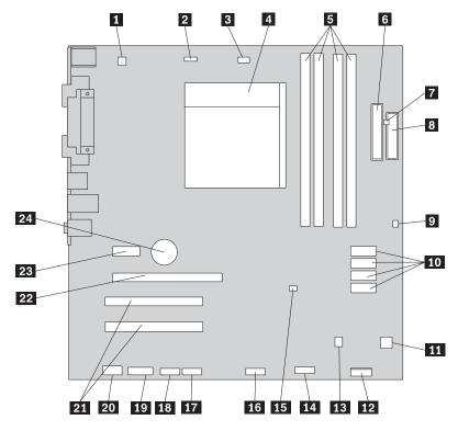
Figure 4. System board parts locations
